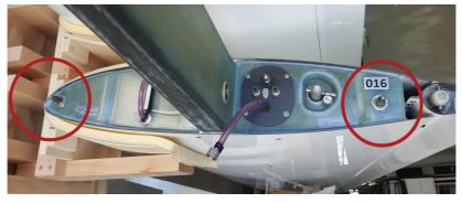
Wing root positioning pins
