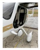
Fuselage mounted towing mirrors
