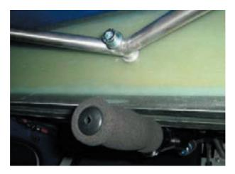
Central wing spar bolt - installed
