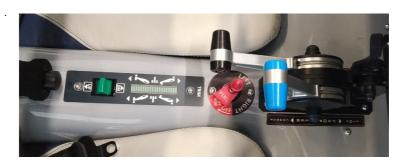
Typical center console arrangement (view of: throttle quadrant, fuel selector, elevator trim, flap lever)
