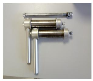
Central spar bolt and two spar pins
